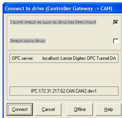
Activate the search process by pressing the **Connect** button to establish an online connection to the drive.
