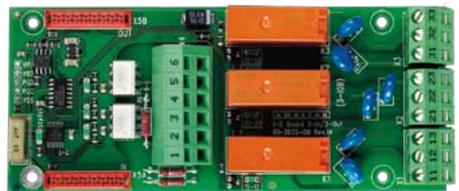
The compact option boards are easily mounted and allow you to combine different options, for example fieldbus communication, motor protection and multiple pump control.
