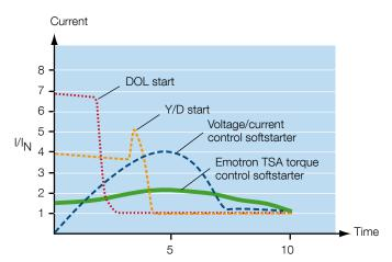
With an Emotron TSA the start current is up to 30% lower than with a conventional softstarter.
