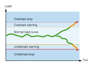
A built-in load monitor protects your process against damage and inefficiency by sending a warning or stopping the process at your chosen load levels.
