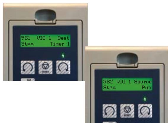
*Emotron VFX supports the virtual connection of logical functions, comparators and timers. The destination and source of a virtual connection can be set easily using the control panel.*
