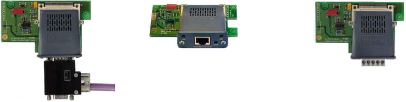
Fieldbus communication, Industrial Ethernet communication and serial communication are supported.
