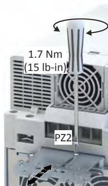
**Installation of shield connection sheet for motor cable 30 kW to 45 kW**
