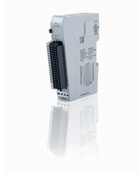
B-Nimis MC-BK DI 16 / DO 16 MC bus coupler with 16 digital inputs and 16 digital outputs.
