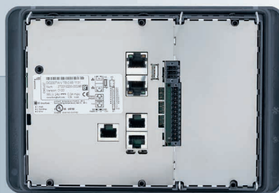
Berghof DC-Pro 7" Display Controller with second CAN bus interface
