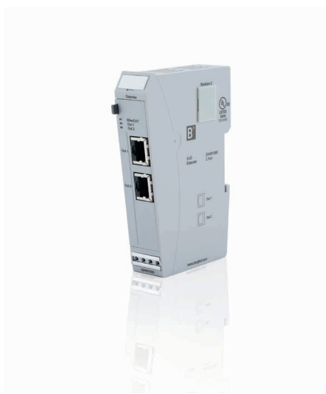
B-Nimis MC-Extender 2 Port The Extender is used to extend E-I/O blocks with additional EtherCAT devices which do not have the MC format. The Extender converts the transmission physics from LVDS (E-bus) to twisted Ethernet.
