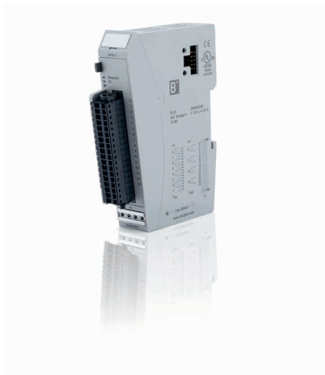
B-Nimis MC-AI4-I 12 Bit CoE* 4 analog inputs for current signals. The measuring range for each channel can be set to 0 ... 20 mA or 4 ... 20 mA .
