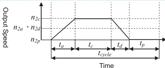
$$ED = \frac{t_a + t_c + t_d}{t_{cycle}}, t_{work} = t_a + t_c + t_d$$
