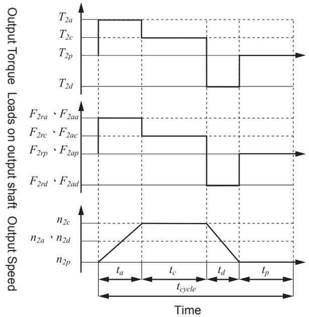
$$\text{Eq.2 } T_{2m} = \sqrt[3]{\frac{n_{2a} \cdot t_a \cdot T_{2a}^3 + n_{2c} \cdot t_c \cdot T_{2c}^3 + n_{2d} \cdot t_d \cdot T_{2d}^3}{n_{2a} \cdot t_a + n_{2c} \cdot t_c + n_{2d} \cdot t_d}}$$
