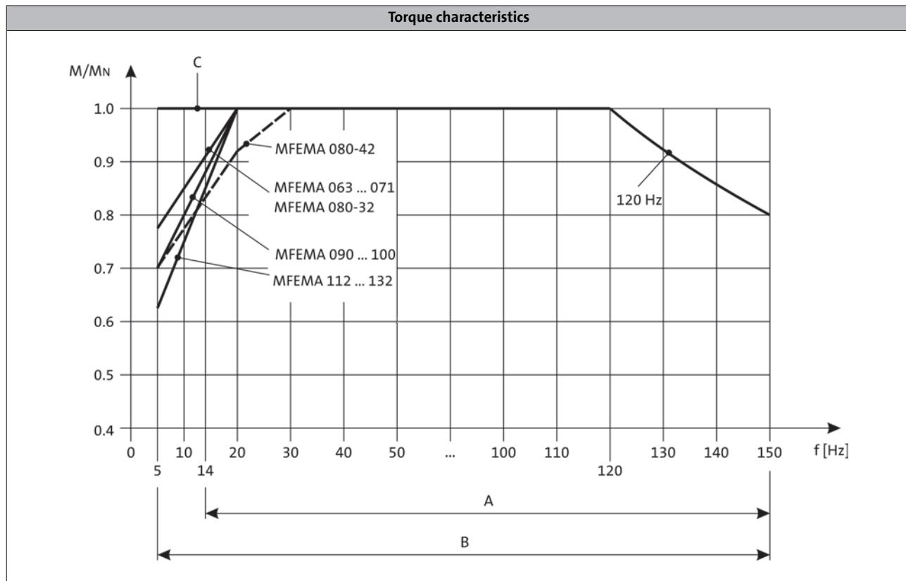
A = Operation with integral fan and brake
