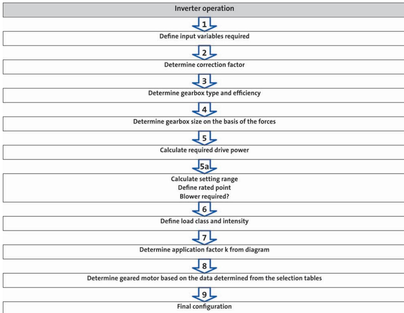
You can use our configuring software Drive Solution Designer for precise drive dimensioning.
