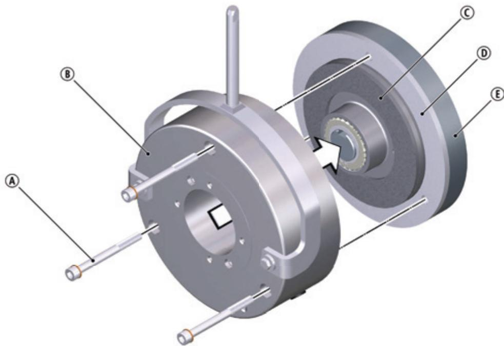
**Fig. 8: Mounting the complete stator**
