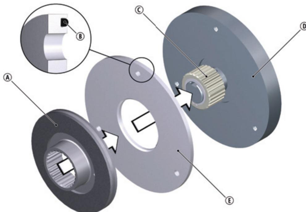
**Fig. 7: Mounting the flange and rotor**
