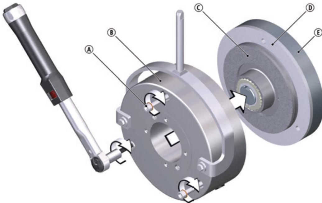
**Fig. 9:** Tightening the screws with a torque wrench
