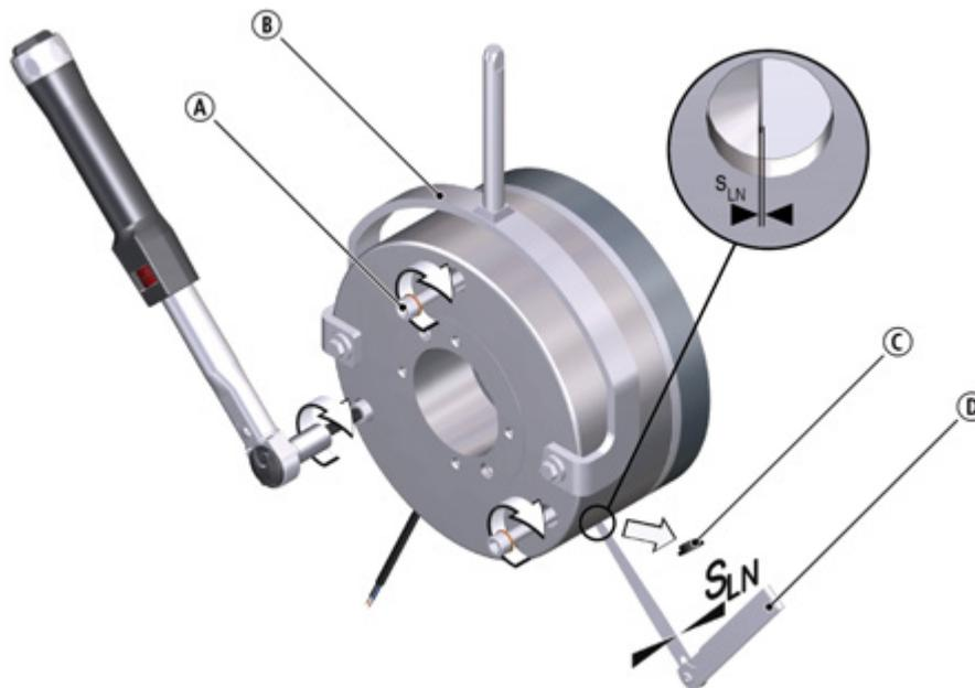
**Fig. 10:** Measure the air gap (for sizes 12 to 18)
