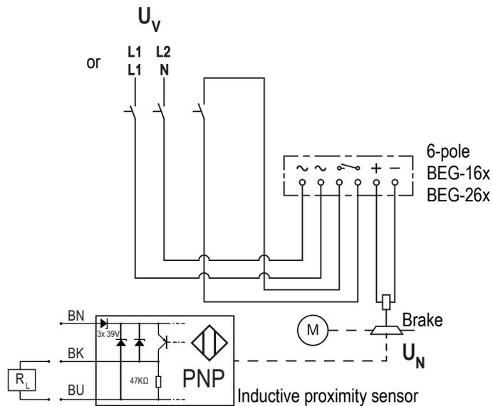
Fig. 18: Supply: Phase-phase or phase-N via 4-pole rectifier
