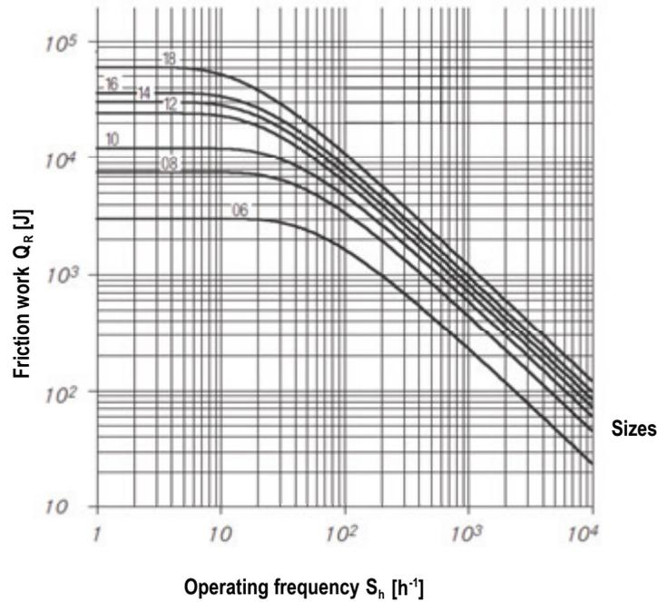
Fig. 3: Friction work as a function of the operating frequency
