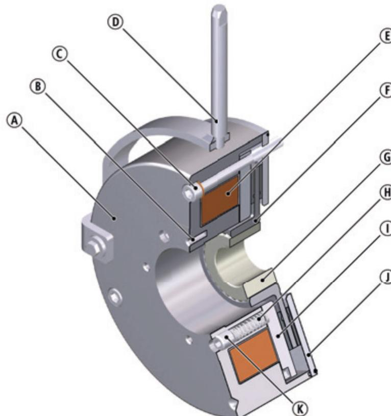
**Fig. 1:** Design of the INTORQ BFK470 spring-applied brake: Complete stator + rotor + flange
