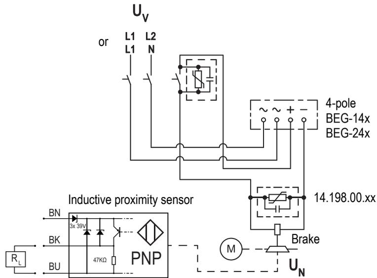
Fig. 17: Supply: Phase-phase or phase-N via 6-pole rectifier
